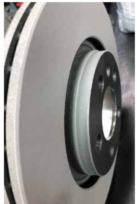
Brake disc with high performance cold gas coating after grinding.
