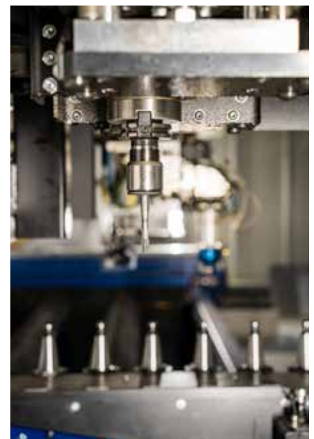
Both machines are equipped with a drilling unit including 24 tool changer.
