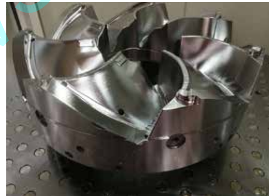
Finished, diffusion-welded tool insert. (Picture: FKT)
