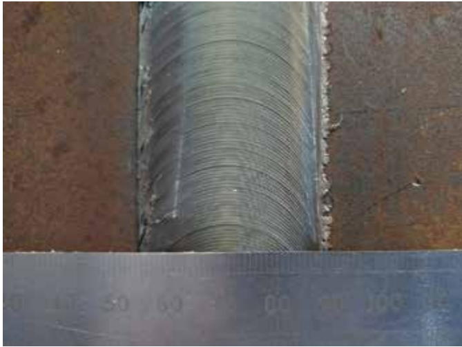
Fig. 3 • Surface detail of a friction stir weld in 12 mm thick S460 steel.
