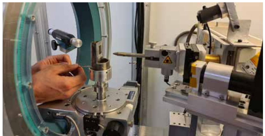
Test lab: Positioning of a sample in the X-ray diffractometer. (Photo: Paul Diekhoff, TU Braunschweig)
