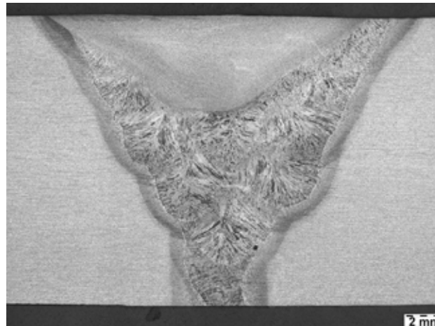
Fig. 6 • A metallographic section through a multi-pass arc weld in 20 mm thick carbon steel, with the weld cap re-processed by FSW to show the difference in weld microstructure. The FSW has a fine microstructure close to that of the parent metal, whereas the arc weld has a coarse, cast microstructure.
