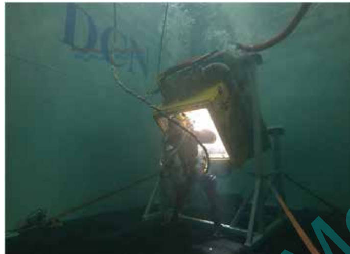
Fig. 11 • "μ-Habitat" factory acceptance test (FAT) / mock-up trials.
