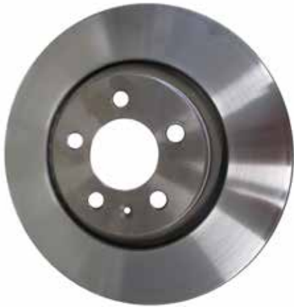
Brake disc with high performance cold gas coating after grinding (Photos: Impact Innovations GmbH).
