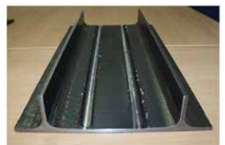
Fig. 5 • Concept of stiffened panel construction from rolled T sections spaced apart with rolled plate (left); integrally stiffened plate demonstration piece fabricated by friction stir butt welding two rolled T sections to a steel plate.
