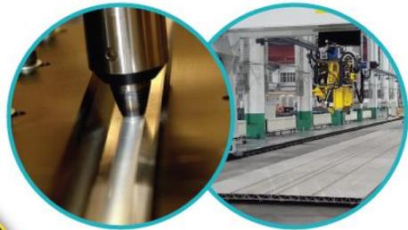
Friction Stir Welding is mechanised, low-distortion, safer welding solution; applicable to (modular) fabrication and underwater repair
